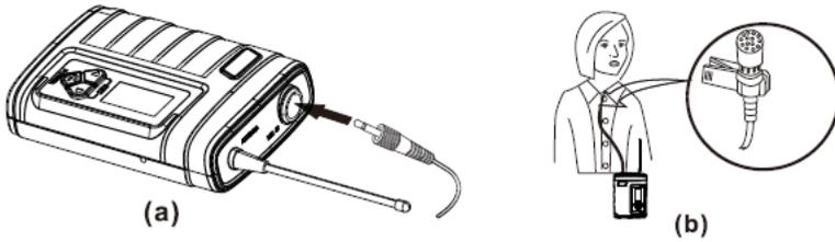
2. Headset Microphone Connection: Connect the connector of supplied headset microphone to the connecting jack of transmitter (Shown as below). Set the transmitter work state in wireless headset system.
