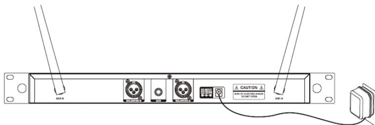
2. Antenna: Keep the position of antenna at a 45 angle from vertical (Shown as below ).
