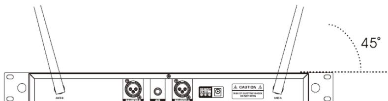
3. Audio Connection: Connect the audio cable from the audio output on the receiver to the input on your amplifier equipment.
