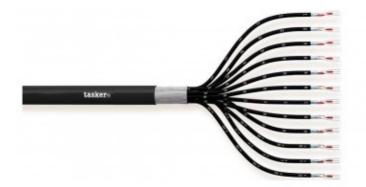
Digital audio multipair cable 110 Ohm AES / EBU -16x2x0.14 mm APPLICATIONS Audio mixers, banks and balanced audio patches
