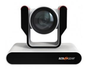
BG-ADAMO-JR is a brand new Full HD PTZ camera with 3 types of lenses available: 12X optical zoom with FOV 70.3, 20X optical zoom with FOV 60.04 and 30X optical zoom with FOV 58.1. It features smooth PTZ functions, advanced image processing features, and flexible connection options.
