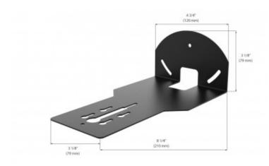
BG-VPTZ-WM is a wall mount bracket for the VPTZ camera series. Multiple cutouts allow for versatile mounting options and cable routing. This bracket is made from heavy gauge heavy gauge steel with a powder coated finish and is designed to provide a secure and stable foundation for your PTZ camera. Can be mounted directly to plasterboard, wood or masonry.
