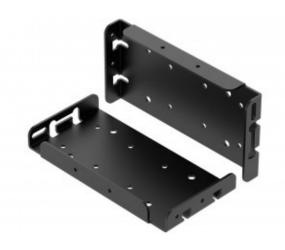
BG-VPTZ-CM is a ceiling mount bracket for BZBGEAR's VPTZ series cameras. It is a slim profile mount designed to secure the camera to the ceiling. The mount has multiple holes for versatile mounting options. It is constructed from heavy gauge steel and covered in a powder coated finish. This bracket mounts directly to drywall, masonry or wood.
