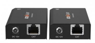
BG-USB-LR100 extends the USB 2.0 port of the PC to distances up to 100 meters with a data transfer rate of up to 480 Mbps through a network cable.
